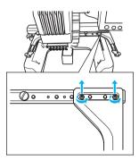
Remove the right arm, align the pins on the embroidery frame holder with the holes in the arm, as shown in the illustration, and then insert the screws removed in step ② and tighten them.
